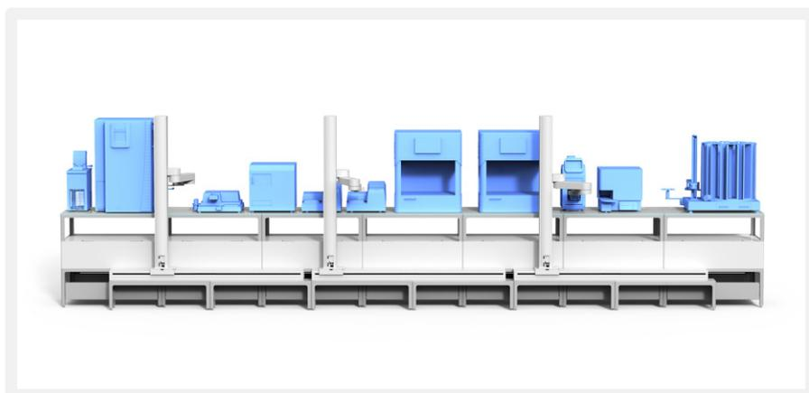
The Automata LINQ system used to fully automate the ELISA workflow
